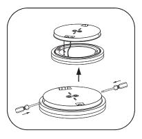
Unlock illuminator from Lamp body: -Push the unlocking-button with standard screw driver
