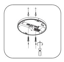
Fix lamp body to the ceiling/wall: -Insert the plastic plug into the pre-driled holes. -Put the mans cable through the cable inlet -Fix the lamp body on to the ceiling/wall with the self tapping screw.
