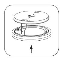
Install the illuminator to lamp body: -Hock the safety cable -Position the illuminator -Push the illuminator into lamp body -Check if the illuminator is safely locked
