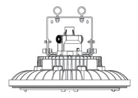
Step4: Use M6 size lifting eye to install on U-bracket.
