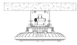
Step4: Use a wrench to tighten the expansion screw.
