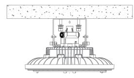
Step3: Align the mounting holes of the CES-EX-GB U-shaped bracket with the holes of the expansion screw.
