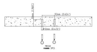
Step1: Open two holes in the wall according to the size in the picture.
