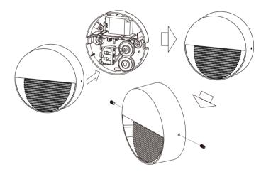
Fix the cover with side cap screws.
