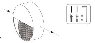
Remove the side cap screws with a hex wrench, then open the cover.
